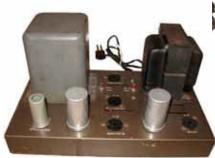
Eico HF-50 Audio Amplifier – The power output from this mono block audio amplifier was 60 watts. Output tubes are 2 x EL34. Made in 1959. The HF-50 used a Chicago output transformer and the HF-60 used a Accrosound output transformer with an output of 60 watts. Karl Breen, Fargo, ND
