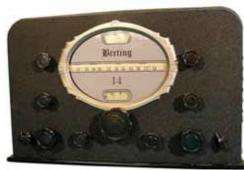
**Bretting model 14** – Manufactured in 1937. The frequency coverage is from 550 kc to 34 mc. It has 14 tubes and originally sold for \$100. Rudy Gertz, Omaha, NE
